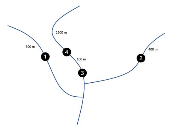
Figure 2. Schematic demonstrating how sets of barriers can be evaluated during prioritization. Barrier 3 would not rank highly, but its remediation is necessary to achieve gains through the remediation of barrier 4. In this case, the set of barriers 3 and 4 would be prioritized above the combination of barrier 1 and 2 as individual barriers.
