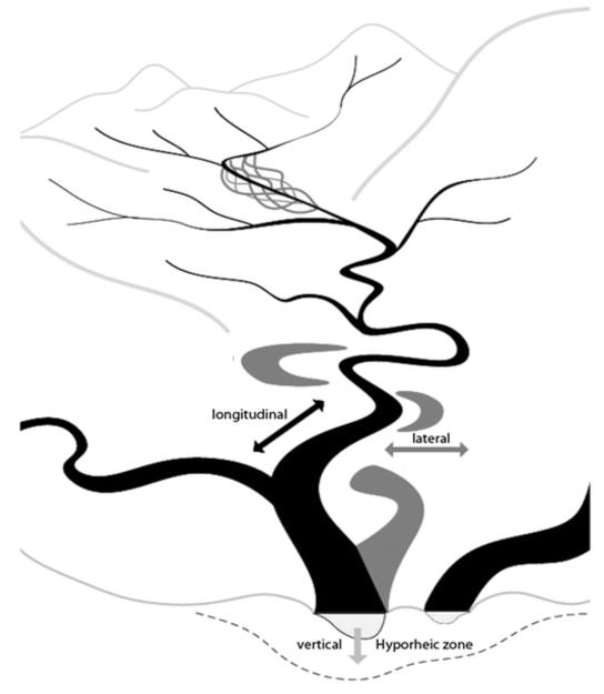
*Figure 1.* An illustration of the three spatial dimensions of freshwater connectivity. Adapted from Seliger and Zeiringer 2018 (<u>CC BY 4.0</u>).
